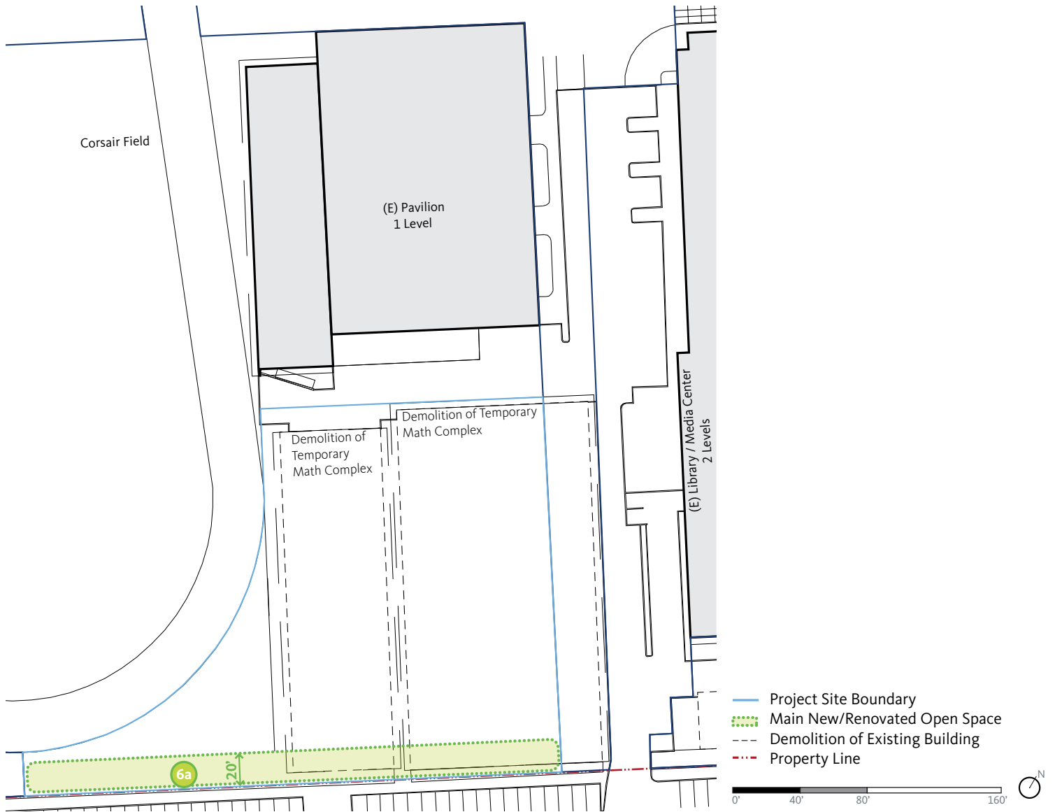
Exhibit 4.43 Project Criteria - Temporary Math Complex Demolition
